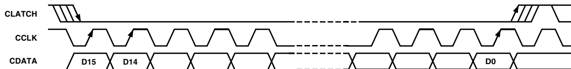
Figure 1. Format of SPI Signal
