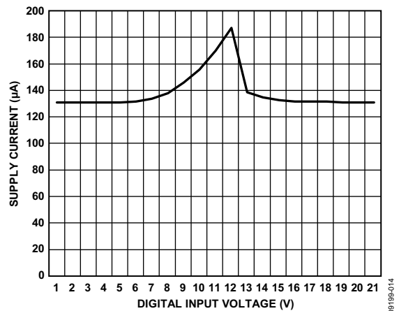
Figure 15. AD5512A/AD5542A Supply Current vs. Digital Input Voltage
