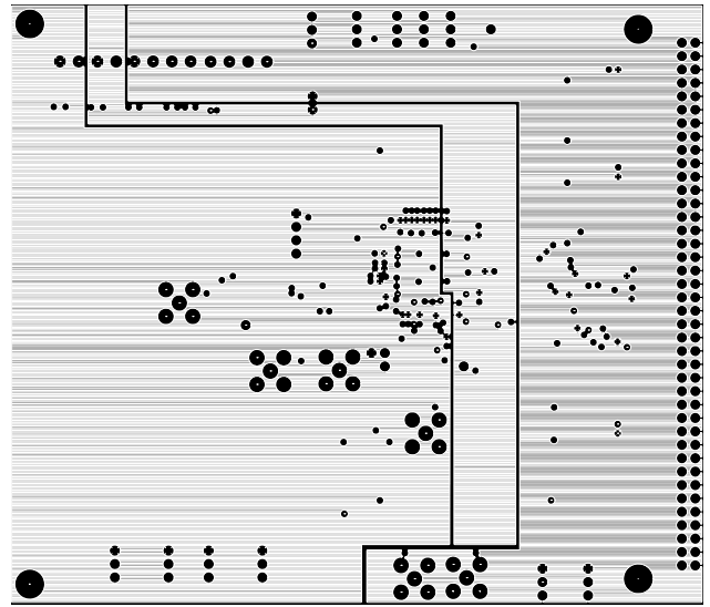
Figure 21. PCB Split Power Plane
