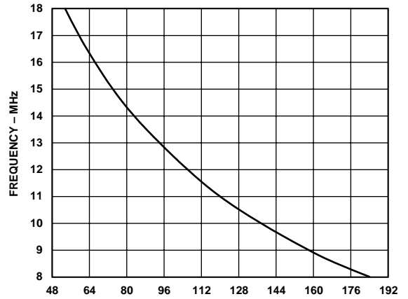
TPC 19. f_c vs. Tuning Target, f_{ADC} = 32 MHz, LPF with Wideband Rx LPF = 0
