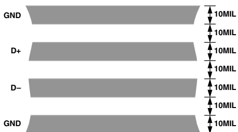
Figure 15. Arrangement of Signal Tracks
