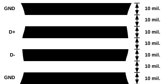
Figure 10. Arrangement of Signal Tracks
