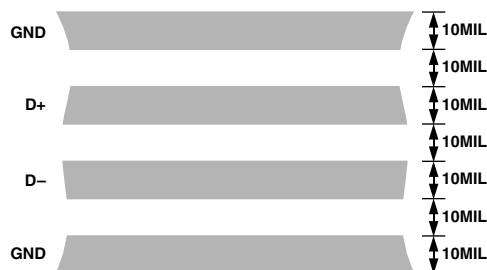
Figure 4. Arrangement of Signal Tracks
