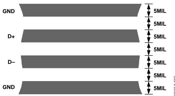
Figure 24. Typical Arrangement of Signal Tracks
