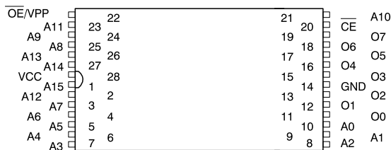
TSOP Top View Type 1
