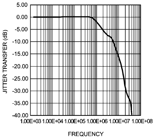
FIGURE 8. Jitter Transfer Curve
