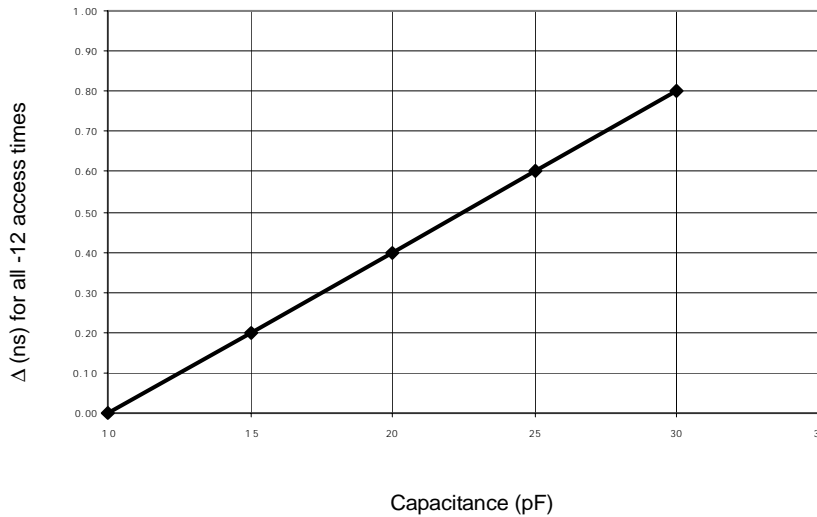
(b) Load Derating Curve
