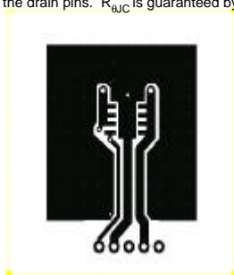
a) 40^\circ\text{C/W} when mounted on a 1\text{ in}^2 pad of 2 oz copper
