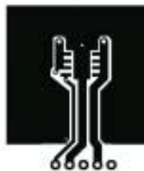
a) 40^\circ\text{C/W} when mounted on a 1\text{ in}^2 pad of 2 oz copper
