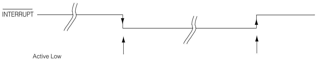
Fig. 2b Reset and Interrupt Timing
