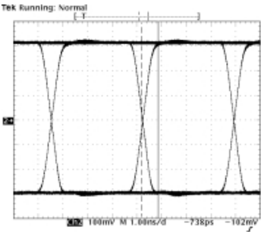
Fig. 3 270Mb/s Eye Diagram
