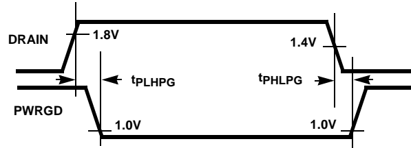
FIGURE 4B. DRAIN TO \overline{\text{PWRGD}} TIMING (ISL6150)
