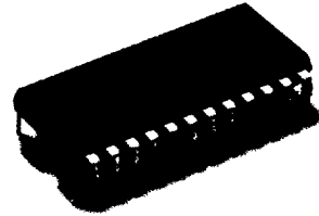
Outline 24P4(P) 2.54mm pitch 600mil DIP (13.0mm × 31.1mm × 3.8mm)
