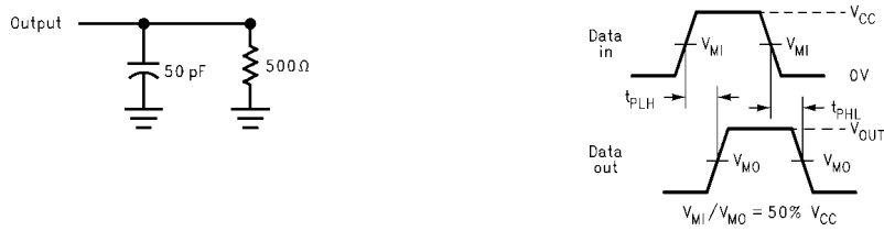
FIGURE 3. t_{PHL} , t_{PLH} Test Load and Waveforms B 1 –B 8 to A 1 –A 8 , C 14 –C 17 to A 14 –A 17 , HLH IN to HLH
