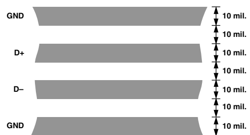
Figure 17. Arrangement of Signal Tracks
