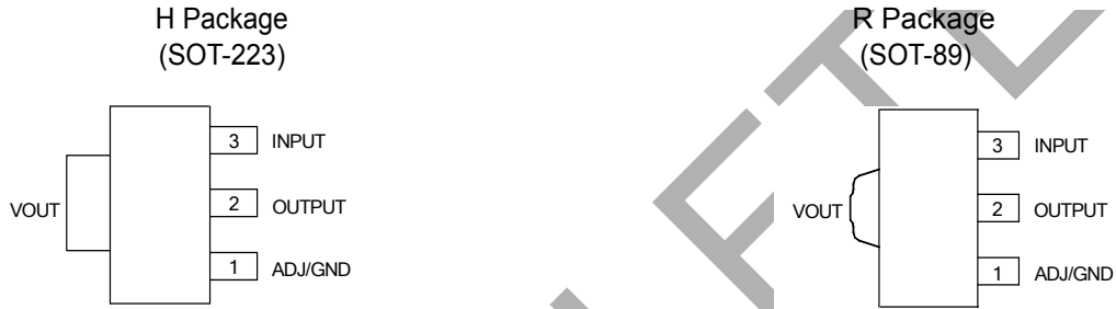
Figure 2. Pin Configuration of AZ1117B (Top View)
