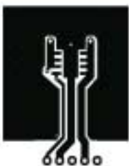
a) 40^\circ\text{C}/\text{W} when mounted on a 1\text{ in}^2 pad of 2 oz copper
