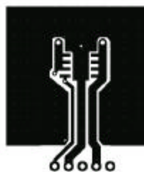
a) 40^\circ\text{C/W} when mounted on a 1\text{ in}^2 pad of 2 oz copper
