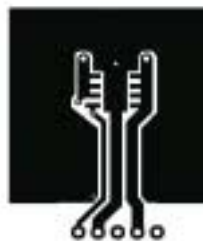
a) 40^\circ\text{C}/\text{W} when mounted on a 1\text{ in}^2 pad of 2 oz copper
