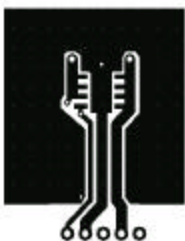
a) 40^\circ\text{C/W} when mounted on a 1\text{ in}^2 pad of 2 oz copper
