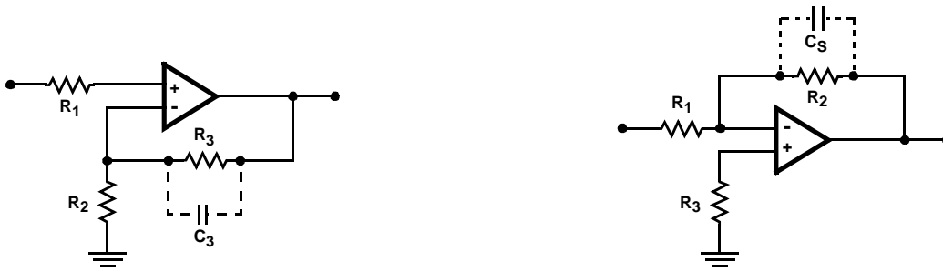
FIGURE 3. SUGGESTED OFFSET VOLTAGE ADJUSTMENT
