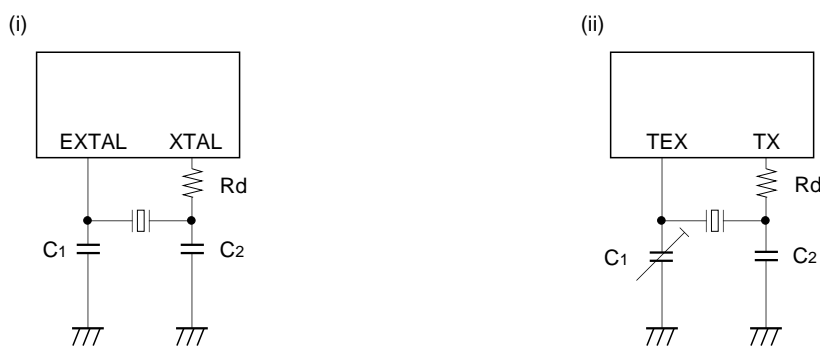
Fig. 13. Recommended oscillation circuit
