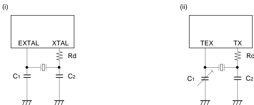
Fig. 13. Recommended oscillation circuit
