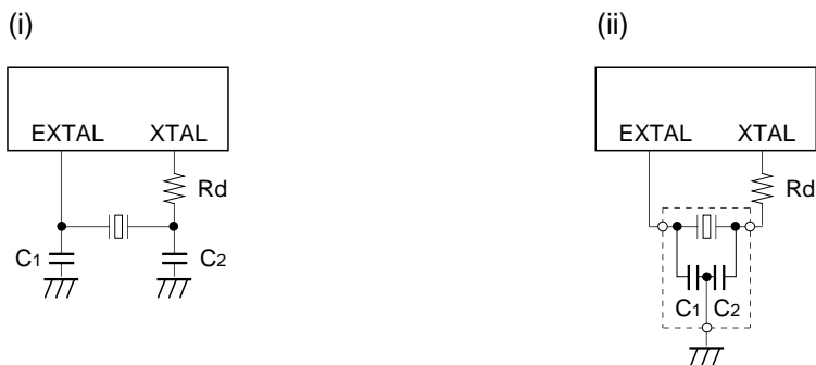
Fig. 13. Recommended oscillation circuit
