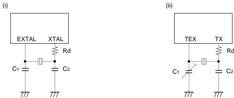
Fig. 11. SPC700 Series recommended oscillation circuit
