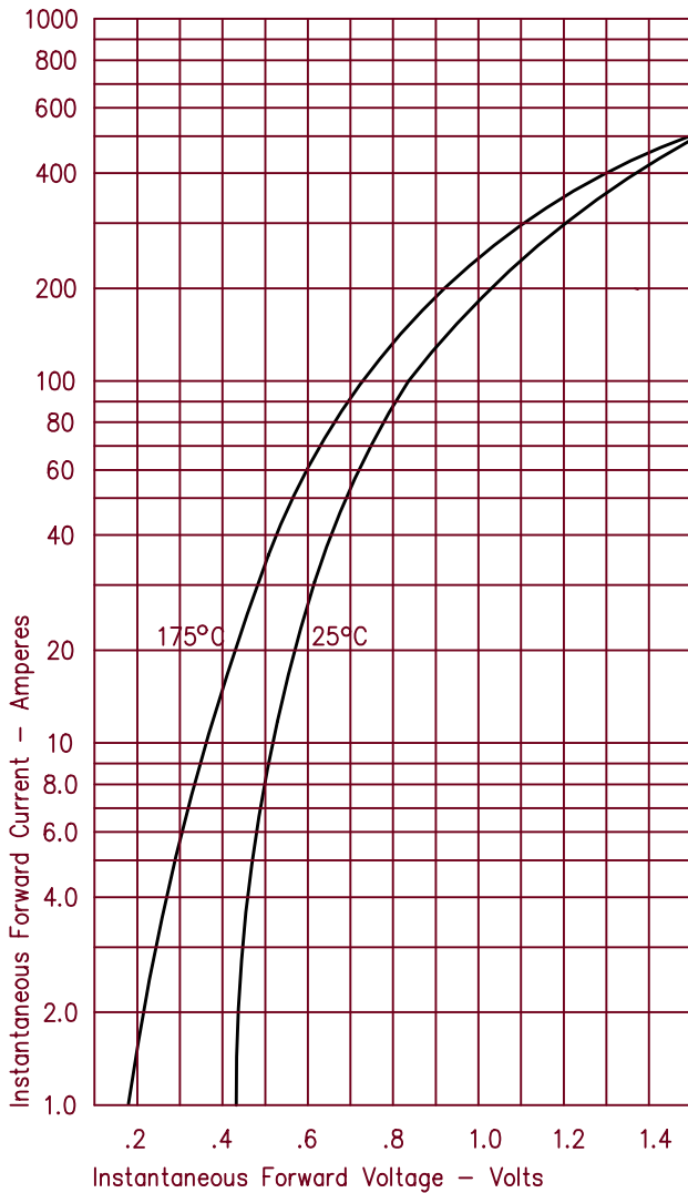
Figure 1 Typical Forward Characteristics
